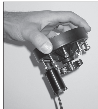
Diaphragm support ring prevents stress failures.
