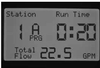
The controller will shut down the station and put it into pause mode for approximately one minute to allow for erratic flow to settle.
