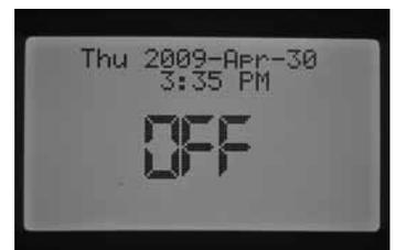
It is also possible to set a programmable period that the controller will remain off in the System Off dial position. This is known as the Programmable Rain Off feature, which will be discussed in the Programmable Rain Off section.
