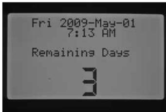
3. Turn the dial back to the RUN position. The display at the RUN position will then show the number of days for the Programmable Rain Off setting. This will count down each day at midnight, showing the remaining days until automatic irrigation will resume.
