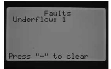
If a flow sensor is selected, stations are set to be monitored, and their flow has been learned, the controller will light the Flow Status light GREEN anytime an acceptable flow is monitored. A flashing RED light indicates an unacceptable flow is occurring.
