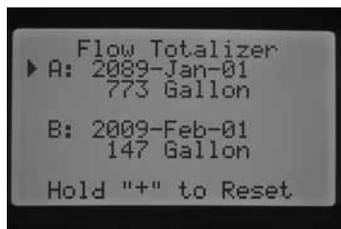
If you would like to reset this reference point, press and hold the + button while the ► cursor is pointing to A. The date will change to the current date, and the gallons will be set back to 0.
