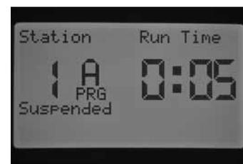
A remote single station command will override the sensor state, whether the station is set to respond or not, and that station will water for the desired run time. When you activate a manual program command by a remote, the controller will acknowledge the stations that have been programmed to respond to a sensor and those stations will not water and be in Suspend Mode.
