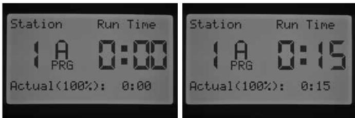
By pressing the PRG button, you can move between programs while staying on the same station. However, it is recommended that one program is completed before going on to the next program.
