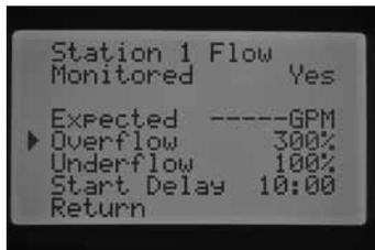
If flow monitoring is enabled for a specific station, the factory preset values will be displayed. The expected flow will be blank, because the actual learning process has not taken place. The learning process will be discussed in the Manual Operation, Learn Expected Flow section. Overflow will be 115%, underflow will be 50%, and the preset Start Delay will be set to 1 minute.
