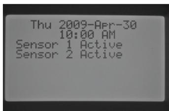
If a station has been programmed to acknowledge the sensor in the SET SENSOR OPERATION dial position, the controller will suspend the watering of those stations.
