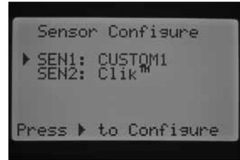
Use the ▲ or ▼ buttons and the ◀ or ► buttons to navigate through the Custom, K-Factor, and Offset screen. Once you navigate to a particular number and it starts flashing, the number may be changed, press the +/- button to either increase or decrease the value. Once you have completed entering the K-Factor and Offset specified by the manufacturer of the flow sensor, use the ▼ button to return to the main Sensor Configuration screen.
