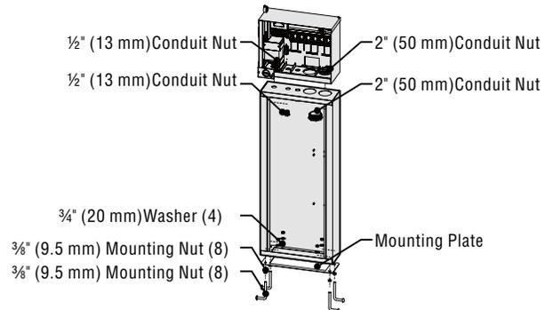
5. Remove the door and faceplate of the I-CORE and attach the metal cabinet of the I-CORE to the top of the pedestal using the enclosed hardware in the pedestal.
