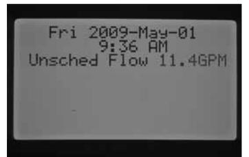
A station not monitored will not be shut down. The controller will detect the flow and determine it as a unscheduled flow.
