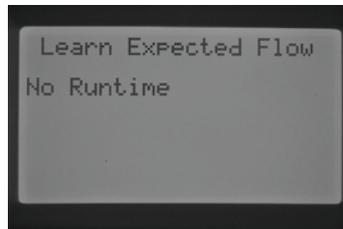
Once flow monitoring has been established, the rules that apply to an overflow or underflow condition are very important to understand. There is a diagnostic testing procedure the controller will activate to determine if there is an overflow or underflow condition. A complete description of the process is explained in the Controller Diagnostics and Troubleshooting section under System Status Dashboard, Flow. It is important to read this section in order to understand the flow monitoring process.
