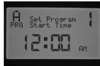
If a program start time is skipped (for example, a start time is set for 1 and 3), the start time will be accepted, but when returning to this dial position, the start times will be moved to sequential order (the Start Time 3 will be moved to 2).
