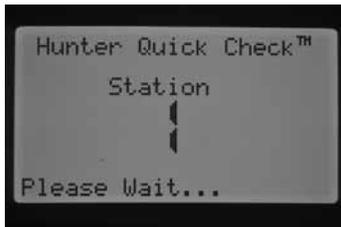
The controller will begin searching all stations in an effort to detect a high current path through the station terminals. If a field wiring short is detected on a station, the controller will display a fault message for each faulty station.
