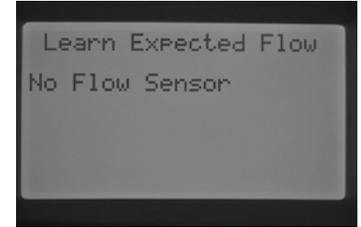
The Learn Expected Flow display will also indicate if there is a problem with any programming. If station run times were not programmed in the SET STATION RUN TIMES screen, the controller will display "No Runtime" in the Learn Expected Flow screen.
