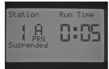
If the controller senses closed circuits across the sensor terminals, the Sensor status light will be GREEN, indicating an Inactive sensor. All programmable watering schedules will proceed as normal.
