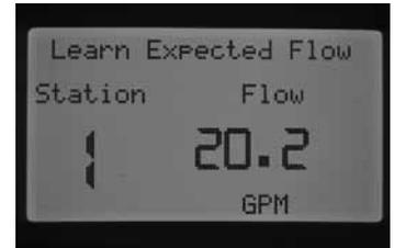
Once the correct station number is displayed, turn the dial to Run. Again, the controller will go into its diagnostic flow testing for that particular station. The controller will activate the station and the learning process may take up to a minute. Once the controller has Learned Expected Flow the controller will shut the stations down and the controller will go back to the main current date / time screen.
