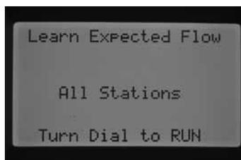
If you want to Learn Expected Flow for All Stations, simply turn the dial to Run. The controller will go into diagnostic testing of the actual flow for each station that has been previously programmed to have its flow monitored. This may take approximately one minute for each station's flow to be learned. It is important to know that during the learning process the station will actually turn on and water in the field.
