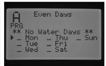
4. In either the Odd or Even Days mode, there will be a \*\*No Water Days\*\* description flashing on the display. Within the Odd or Even mode you can select days that watering will NOT
