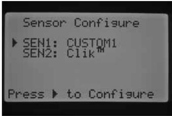
Use the ▲ or ▼ buttons and the ◀ and ▶ buttons to navigate through the Custom, K-Factor, and Offset screen. Once you navigate to a number, it will flash. The number may be changed by pressing the +/- button to either increase or decrease the value. Once you have completed entering the K-Factor and Offset specified by the manufacturer of the flow sensor, use the ▼ button to return to the main Sensor Configuration screen.
