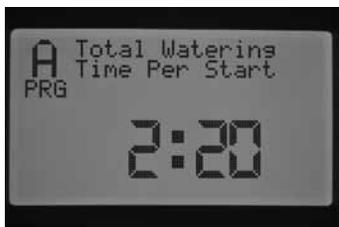
The controller acknowledges which stations have a run time associated with each program, and adds all the station's run times together to equal the total run time or watering duration for that Program. Total Watering Time does not take into consideration any Cycle and Soak and Station Delay times that will occur during irrigation.
