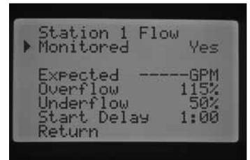
**Expected Flow** – the amount of flow expected for that station in Gallons Per Minute (GPM) or Liters Per Minute (LPM)
