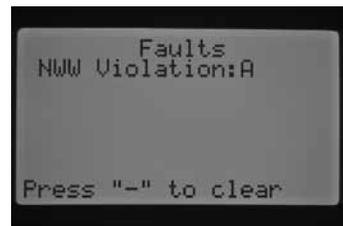
This message is displayed to make you aware that irrigation has been missed or Suspended and supplemental watering may be necessary to make up the missed irrigation that has occurred during the No Water Window. A manual single station that is activated remotely or at the controller will override the No Water Window and be allowed to water.
