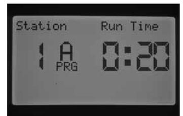
After no more buttons are pressed, the controller will automatically begin watering. After the manual program begins, you may also use the ► button to scroll to a particular station or advance to a station more quickly.
