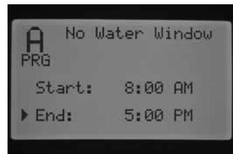
**For example:** if the No Water Window Start is set at 8:00 AM and the No Water Window End is set at 5:00 PM, the controller will not irrigate during the period of the day between 8:00 AM to 5:00 PM.
