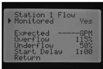
Flow Operation is necessary to program in order for the controller to know which stations to monitor. Important additional steps that need to be taken to complete the flow monitoring setup. A flow sensor needs to be assigned in the Sensor Configuration screen, and the stations set to be monitored need their flows to be learned. These steps are required in order for flow monitoring to occur.
