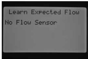
If the user has not selected a station's flow to be monitored the controller will display "No Flow Station," as well as "No Runtime" even if there is a run time associated with the stations.
