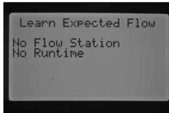
If the user has not programmed station run times in the SET STATION RUN TIMES screen, the display will read "No Runtime."
