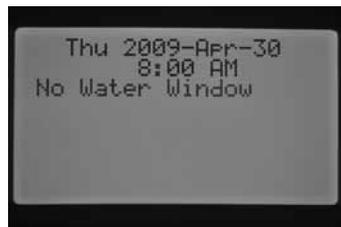
The program will continue to count down the run times associated with the program. If the No Water Window expires and the program is still counting down a run time, the controller will begin watering at that point in time. Once the program finishes and the display returns to the current date and time screen, a fault message will be displayed indicating irrigation has violated the No Water Window and which program was in violation.
