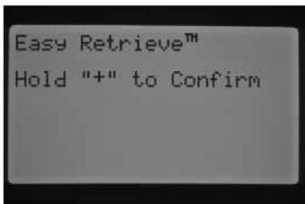
If you erase the controller's memory by using the Erase All feature found in Advanced Features, which will be discussed in a few sections, the controller will revert back to factory presets, and you will NOT be able to retrieve the Easy Retrieved saved programming. The Easy Retrieve program that was saved will be overwritten and lost.
