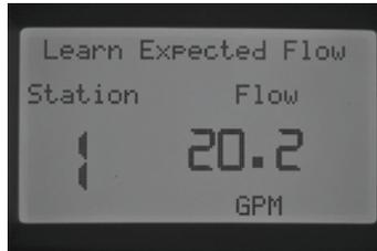
If no HFS FCT size was programmed in the Sensor Configuration section of Advanced Features, the controller will display "No Flow Sensor" in the Learn Expected Flow screen.
