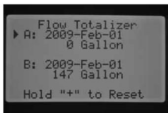
Use the ▼ button to select point B. The ► cursor will be displayed next to point B. To reset reference point B, press and hold the + button, the date will change to the current date and the gallons will be set back to 0.
